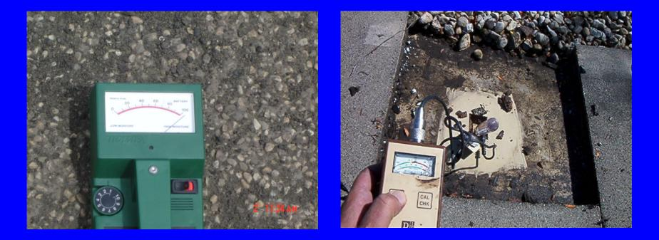
Moisture Meters are used to verify if there is wet insulation at locations indicated by the infrared scan. Cores are taken to determine the type of insulation and the amounts of roofing on the building as well as the deck type and attachments.
